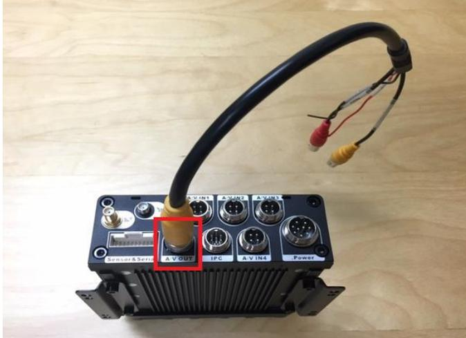
3. XDR Rear – Connect **EX4-NPIG** to **AV-OUT** port on XDR for video out connection to monitor. May need BNC to RCA converter
