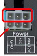
Connect the power cable 6 prong white plug to the VMDR-888 Power connector on the rear.
